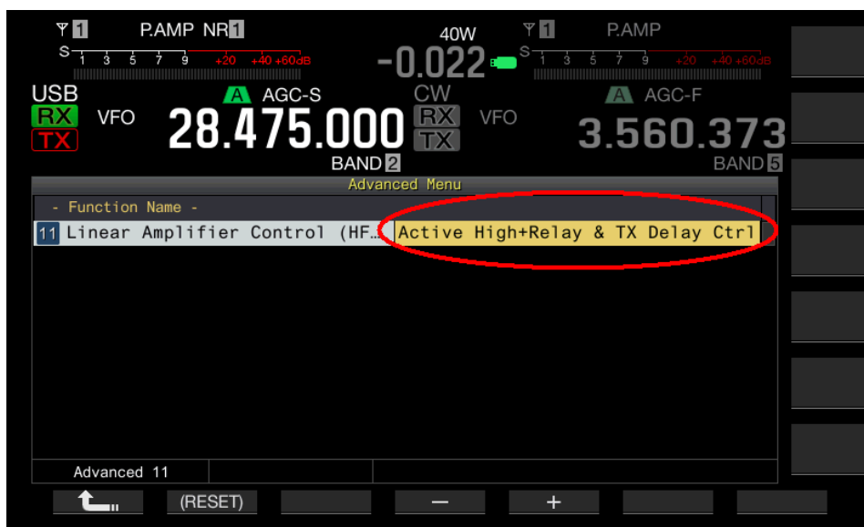
Figure 1: TS-990 Menu Settings for Linear Amplifier Control
