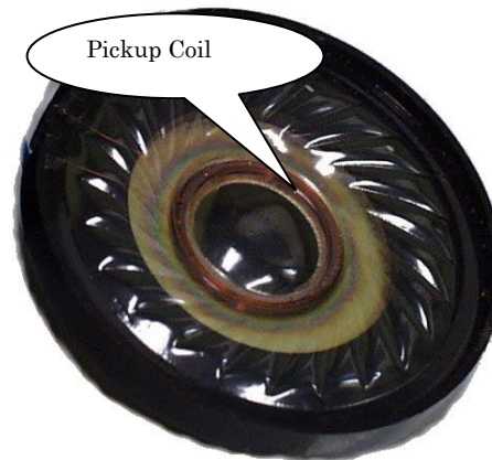
Figure 1-2: A Typical Dynamic Microphone Element
