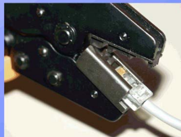
Figure 16-7: How to Install RJ-45 Connectors on UTP Cable
