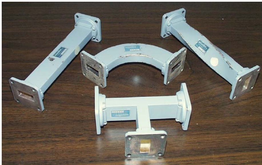
Figure 13-5: Several Types of Waveguide Clockwise, from Upper Left: Straight; H-Bend; Twist; Series Tee
