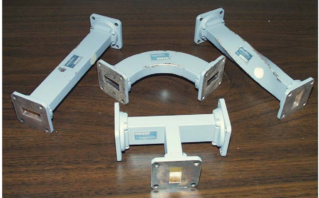
Figure 13-5: Several Types of Waveguide Clockwise, from Upper Left: Straight; H-Bend; Twist; Series Tee
