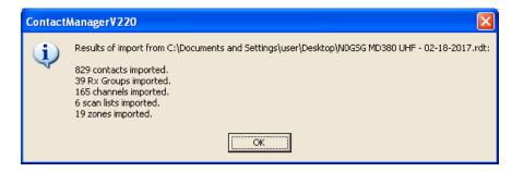
In this instance, we have moved all the data from NØGSG's MD380 codeplug into a CS800 codeplug. The CS800 will have all the contacts, receive groups, channels, scan lists, and zones provided by the MD380 codeplug, and they'll be organized identically.
